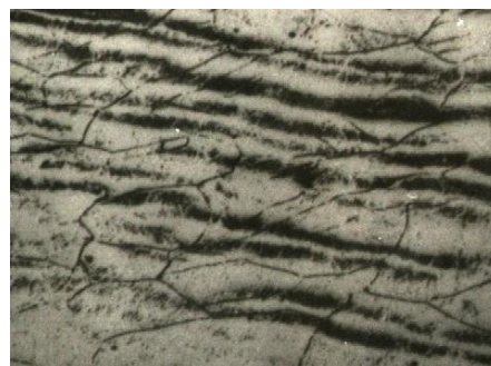
Fig. 4 Microstructure of thermal-treated and vibrated nuts - 200X
