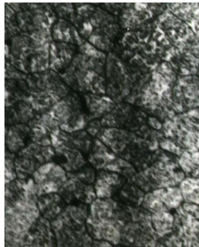
Fig. 6 Microstructure of thermal-treated and vibrated bearings - 200X nital attack
