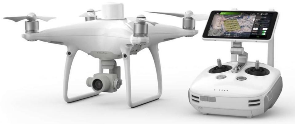
**Fig. 2** DJI Phantom 4 UAV with RTK module (top side) and Controller [9]
