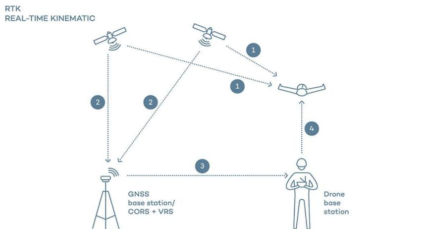
**Fig. 1** Real-Time Kinematic - data transmission [8]
