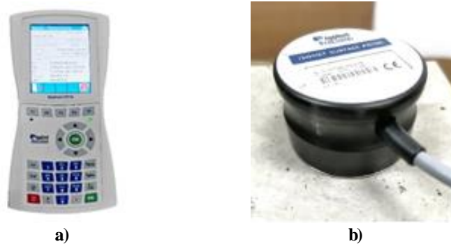
Fig. 3 Measure the thermal conductivity: (a) the display of ISOMET 2114; (b) the measuring device for hard surface
