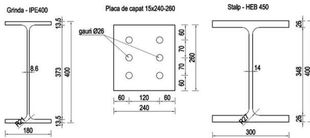
Fig. 4 Components of the Verified Joint
