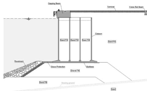
Quay wall made of floating caissons
