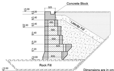
Quay wall made of hollow blocks
