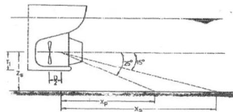
**Fig. 6** Calculation elements for the jet contact zone with the bottom of the basin
