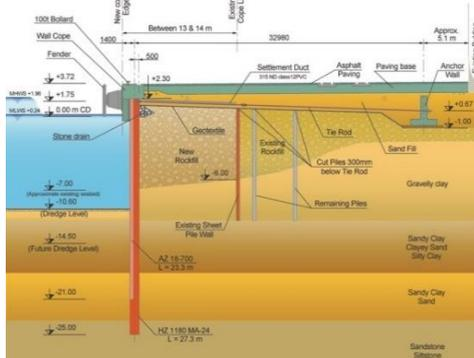
Quay wall made of steel sheet piles
