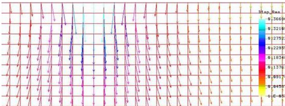
Fig. 9 Vector diagram of the resulting displacement obtained using the COSMOS/M program for a pressure of 5 kPa
