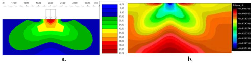
**Fig. 10** Stress diagrams  $\sigma_x$  [kPa]: a. GEO5 – FEM for a pressure of 180 kPa, b. COSMOS/M for a pressure of 250 kPa
