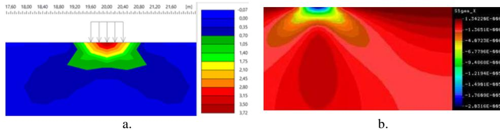
**Fig. 5** Stress diagrams  $\sigma_x$  [kPa] for a pressure of 5 kPa: a. GEO5 – FEM, b. COSMOS/M
