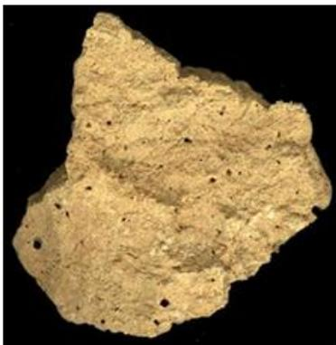
**Fig. 1** Macroporous loess from Constanța's seafont [2]
