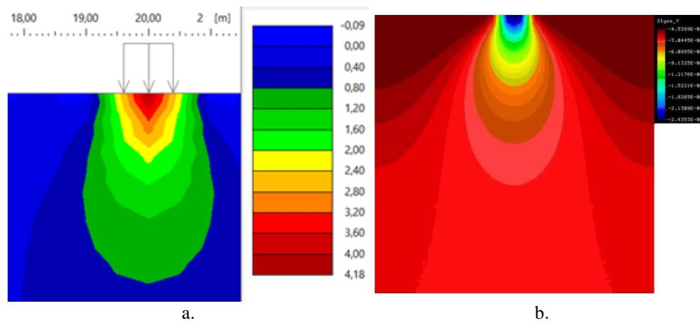
**Fig. 6** Stress diagrams  $\sigma_z/\sigma_y$  [kPa] for a pressure of 5 kPa: a. GEO5 – FEM, b. COSMOS/M
