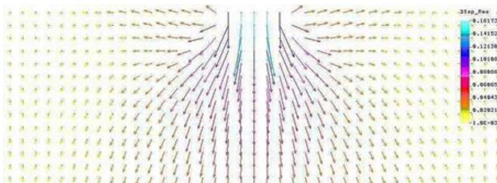
Fig. 15 Vector diagram of the resultant displacement obtained using COSMOS/M for a pressure of 250 kPa
