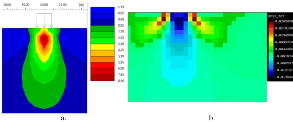
Fig. 13 Specific strain diagrams  $\epsilon_z / \epsilon_y$  [%]: a. GEO5 – FEM for a pressure of 180 kPa, b. COSMOS/M for a pressure of 250 kPa
