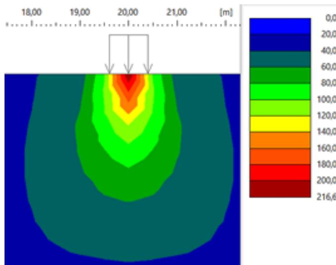
Fig. 14 Displacement diagram  $d_z$  [mm] obtained using GEO5-FEM for a pressure of 180 kPa
