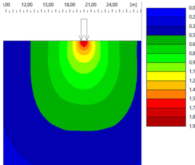
Fig. 8 Displacement diagram  $d_z$  [mm] obtained using GEO5-FEM for a pressure of 5 kPa
