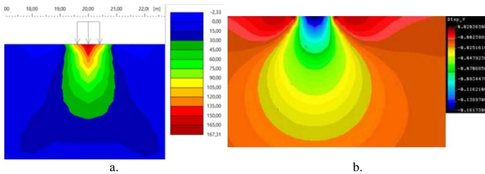
**Fig. 11** Stress diagrams  $\sigma_z / \sigma_y$  [kPa]: a. GEO5 – FEM for a pressure of 180 kPa, b. COSMOS/M for a pressure of 250 kPa
