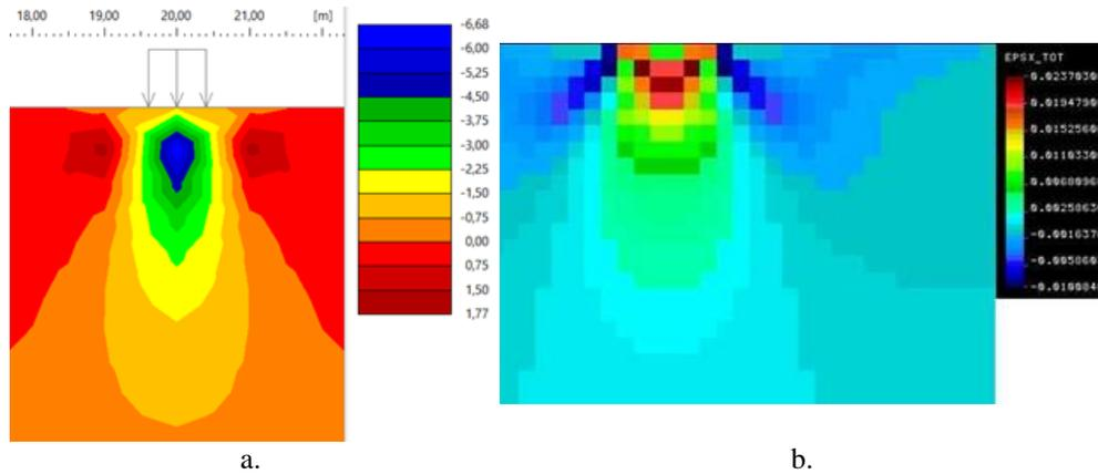
**Fig. 12** Specific strain diagrams  $\epsilon_x$  [%]: a. GEO5 – FEM for a pressure of 180 kPa, b. COSMOS/M for a pressure of 250 kPa
