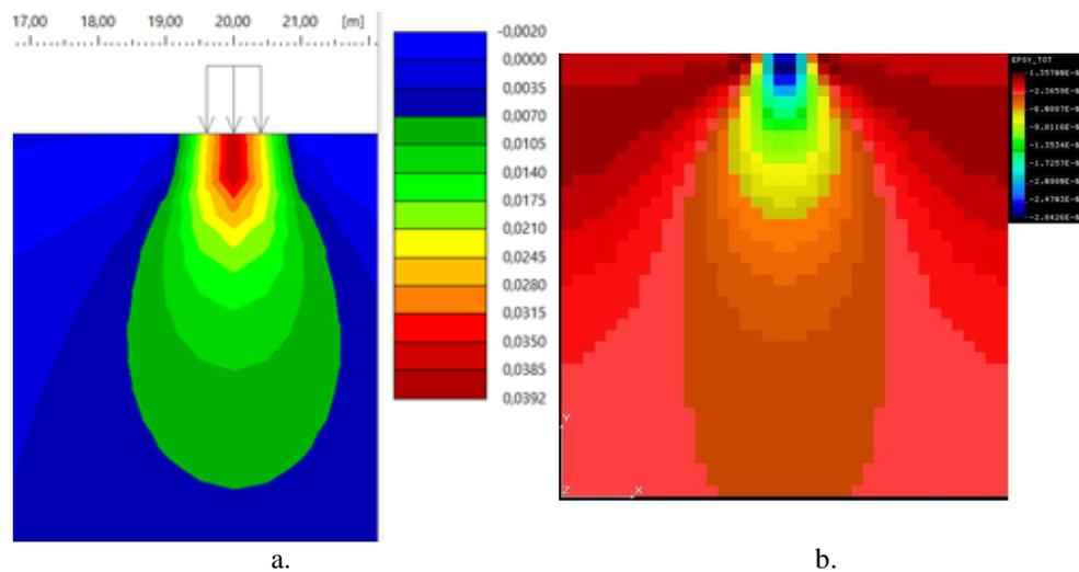
**Fig. 7** Specific strain diagrams  $\varepsilon_z/\varepsilon_y$  [%] for a pressure of 5 kPa: a. GEO5 – FEM, b. COSMOS/M
