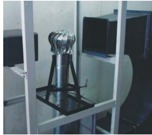
Fig. 2. Axonometric view of the used wind tunnel with a detail of the test chamber with wind turbine
