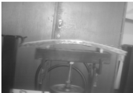
Fig.9. Composite sample showing considerable deflection without cracking
