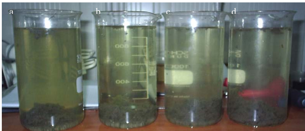
Fig. 1. Coagulation – flocculation process using a cationic flocculant and iron(III) sulfate 42% in different doses: a – 500 µl/l; b – 600 µl/l; c – 700 µl/l; d – 800 µl/l.
