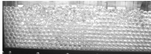
Photo 4. Glass spheres laying in a transparent canal (down-part tetrahedron, up-disorderly laying)
