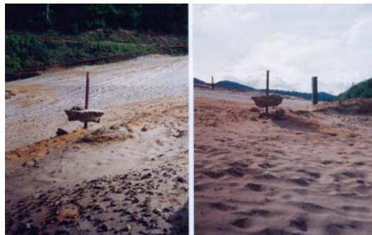
Fig. 5 – Topographic marks on the bank of Valea Târnicioara decantation pool
