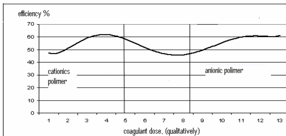
Fig. 4. Coagulation – flocculation zones depending on the coagulant concentration
