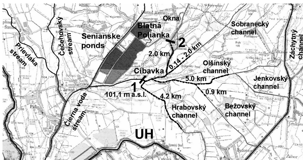
Fig. 3. Simulated back water after the crest increasing on the Cibavka weir
