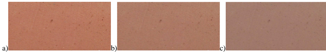
Fig. 4. a) chromatic of the dried sample, b) chromatic of the sample with 10% water, c) chromatic of the sample with 20% water.
