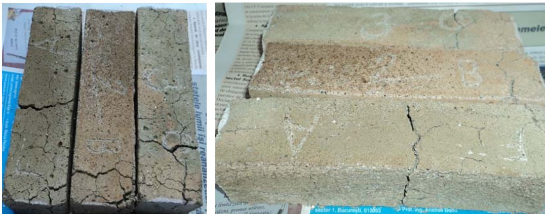
Fig. 3 Sand concrete samples fired at 1600°C
